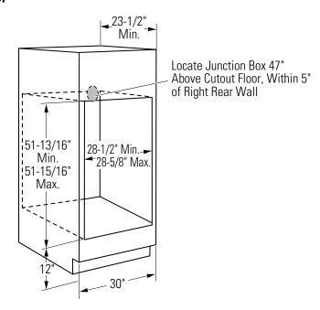
The solid bottom or runners must be level with the bottom of the cutout, or the bottom trim may not install correctly and could interfere with the door opening. If the cabinet does not have a solid bottom, two braces or runners must be installed level with the bottom of the cutout to support the weight of the oven. The runners and braces must support 300 lbs. (135 kg).
